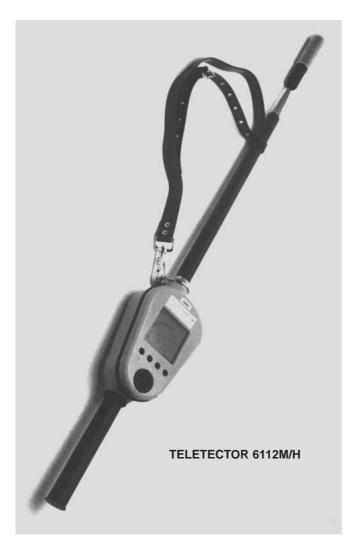
The Teletector 6112M/H is a portable battery operated dose rate meter to measure photon radiation (gamma and X-radiation), and to detect beta radiation. Two GM counter tubes serve as detectors. The stainless steel telescope can be continuously extended up to more than four metres; its tip carries the two tubes. The tubes are placed along the axis one behind the other; a groove marks the centre of each tube. The
