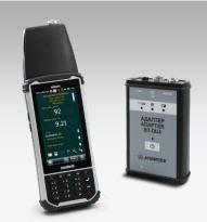
2) PU4 is a hand-held PC (HPC) with integrated detection module, providing in situ measurement of gamma radiation dose and dose rate. Operation algorithm provides measurement continuity and real time statistical processing of measurement results.
