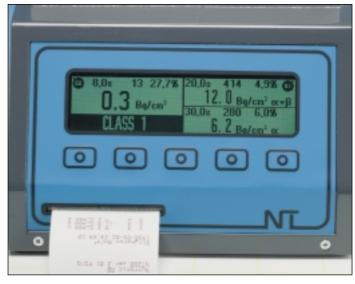
A measurement in auto-alpha mode with the NT200. In the right windows alpha activity has been registered. The display clearly indicates this and shows the alpha and beta results separately.
