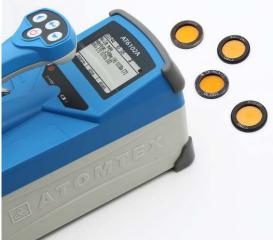
The possibility of external detection unit connection allows measurement of alpha and beta particles flux density from contaminated surfaces (BDPA-01/BDPB-01) and neutron radiation dose rate (BDKN-03).
