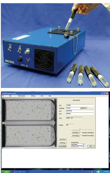
The **BDR-III™ Automatic Bubble Reader** is an affordable solution for automatic counting of large numbers of detectors. The BDR-III provides bar code-ready, fully automated counting with machine vision technology that generates database compatible files in a compact, simple-to-use instrument.
