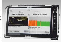
When radioactive source is detected the system activates alarm and identifies its radionuclide composition.
