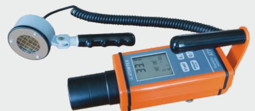
The Radiation Monitors can be delivered with an external BDPS-02 detection unit, designed for measuring alpha and beta particle flux density from flat contaminated surfaces, gamma and X-radiation ambient dose equivalent and ambient dose equivalent rate.
