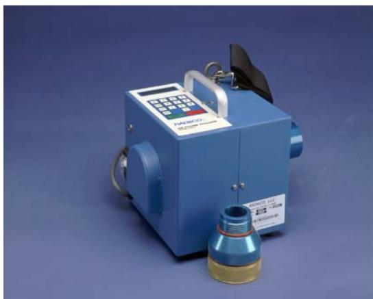
The Model H-810 has been designed using the latest in technology. The unit is microprocessor based with battery backed data memory to store operational parameters for as long as 10 years. All calibrations are performed using the on-board membrane key pad.
