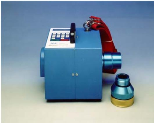
The Model H-810DC has been designed using the latest in technology. The unit is microprocessor based with battery backed data memory to store operational parameters for as long as 10 years. All calibrations are performed using the on-board membrane key pad.
