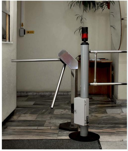
Stationary pedestrian radiation monitor is designed to detect gamma radiation sources continuously and automatically in a stream of people crossing borders of secure facilities.
