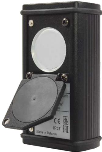
When the filter cap opens the instrument switches to beta particle flux density measurement mode automatically.
