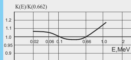
Normal energy relationship between monitor sensitivity and <sup>137</sup>Cs gamma radiation energy of 662 keV
