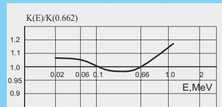
Normal energy relationship between monitor sensitivity and <sup>137</sup>Cs gamma radiation energy of 662 keV
