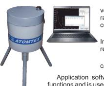
Matrix method allows measurement of volumetric (specific) activity for monitored radionuclides based on energy windows count rate.
