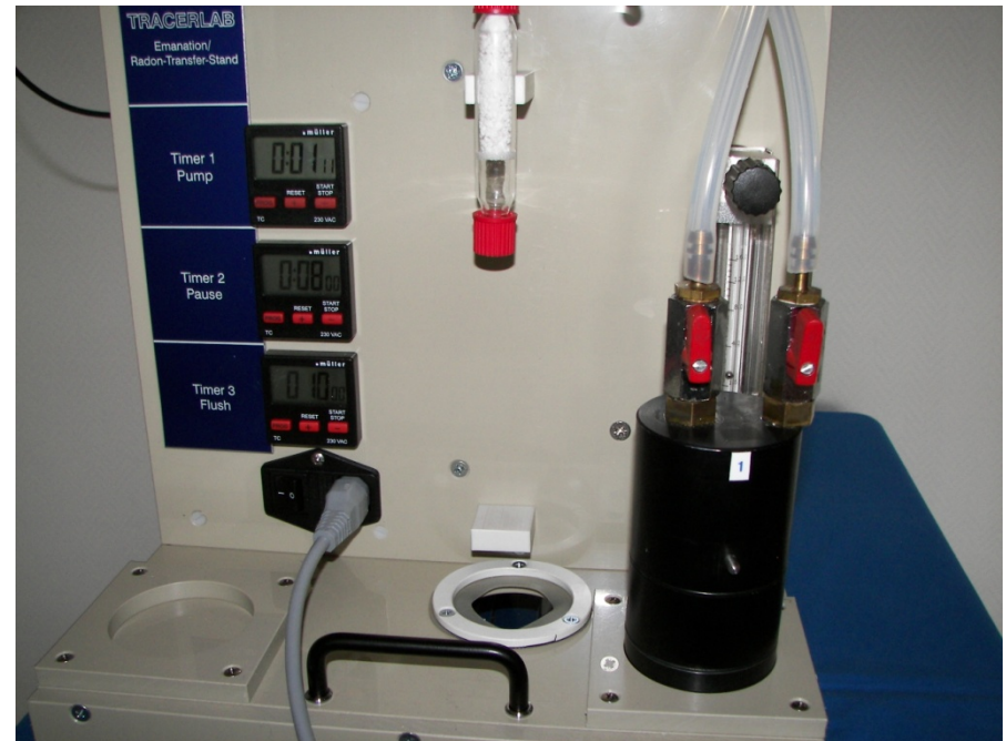
Automatic cleaning process of used scintillation chambers with a timer-controlled program
