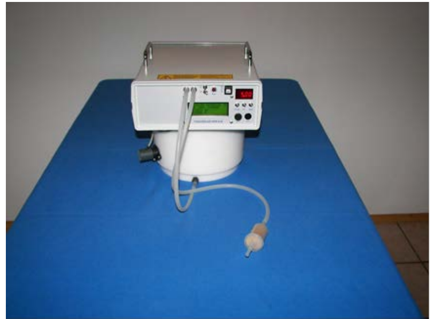
ERS-2-S, standard version with the 4-line LCD, operation by pumping-mode
