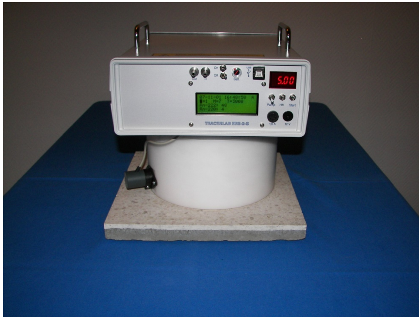
ERS-2-S, standard version with the 4-line LCD, operation by diffusion-mode
