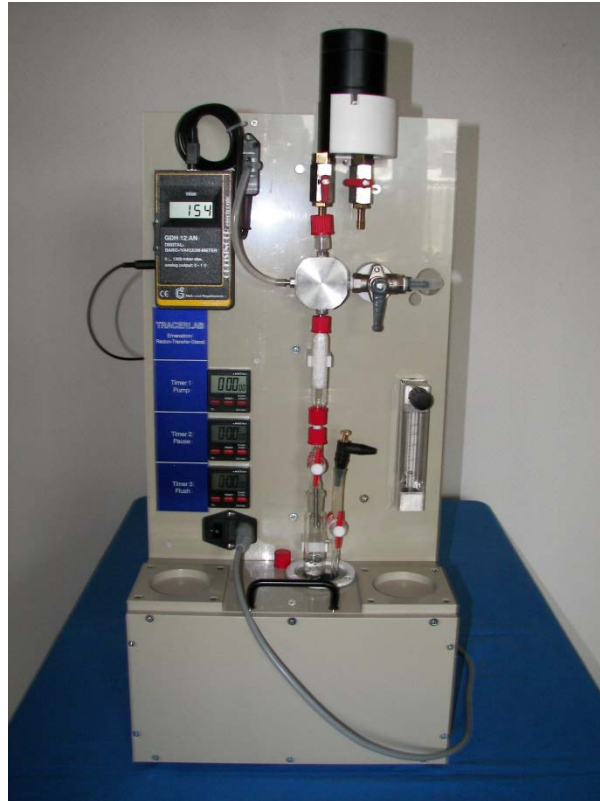
Emanation-Stand for the transfer of the Radon-Gas into the evacuated Scintillation-Chamber
