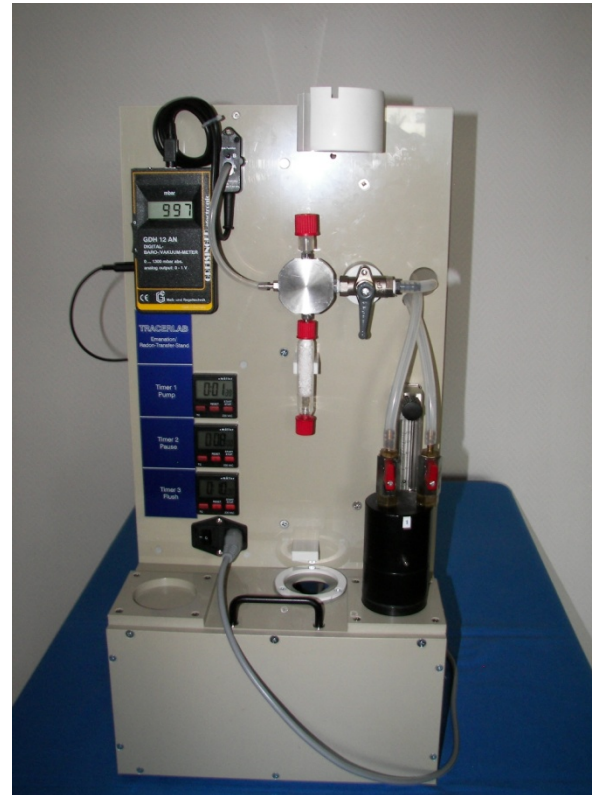
Emanation-Stand with the ACTIVE and timer-controlled cleaning PROCESS
