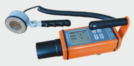
The Radiation Monitros can be delivered with an external BDPS-02 detection unit, designed for measuring alpha and beta particle flux density from flat contaminated surfaces, gamma and X-radiation ambient dose equivalent and ambient dose equivalent rate.
