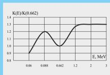
Normal energy response of monitor sensitivity respect to <sup>137</sup>Cs gamma radiation of 662 keV
