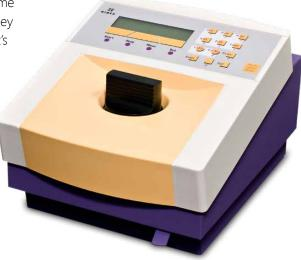
into the field to measure samples on the spot. Although compact, Triathler has many advanced features such as advanced spectrum analysis using a multichannel analyzer (MCA), Instant DPM results, single-photon luminescence counting, and optional alpha beta separation.
